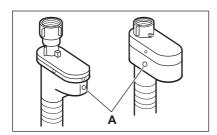
The inlet hose has a water stop device. This device prevents water leaks in the hose because of its natural ageing.
