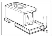
Remove the polystyrene protection from the bottom. Pull up the appliance in vertical position.
