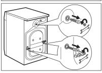
Remove the three bolts. Use the key supplied with the appliance. Pull out the plastic spacers.
