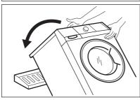
Put one of the polystyrene packaging elements on the floor behind the appliance. Carefully put down the appliance with the rear side on it. Make sure not to damage the hoses.
