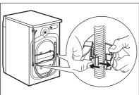
Remove the power supply cable and the drain hose from the hose holders.
