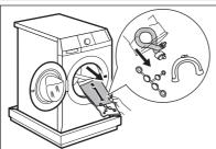
Open the door. Remove the polystyrene piece from the door seal and all the items from the drum.
