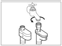
• Connect the water inlet hose to the cold water tap with 3/4 thread.
