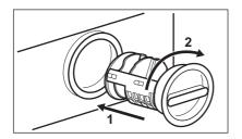
8. Put the cap back on the emergency emptying hose and place the latter back in its seat. Replace the filter into the pump by inserting it correctly into the special guides. Screw the filter cover firmly by turning it clockwise.
