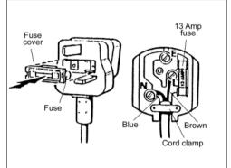
The wire which is coloured blue must be connected to the terminal which marked with the letter N or coloured black.
