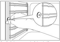
Pull the rear end of the shelf support away from the side wall and remove it.
